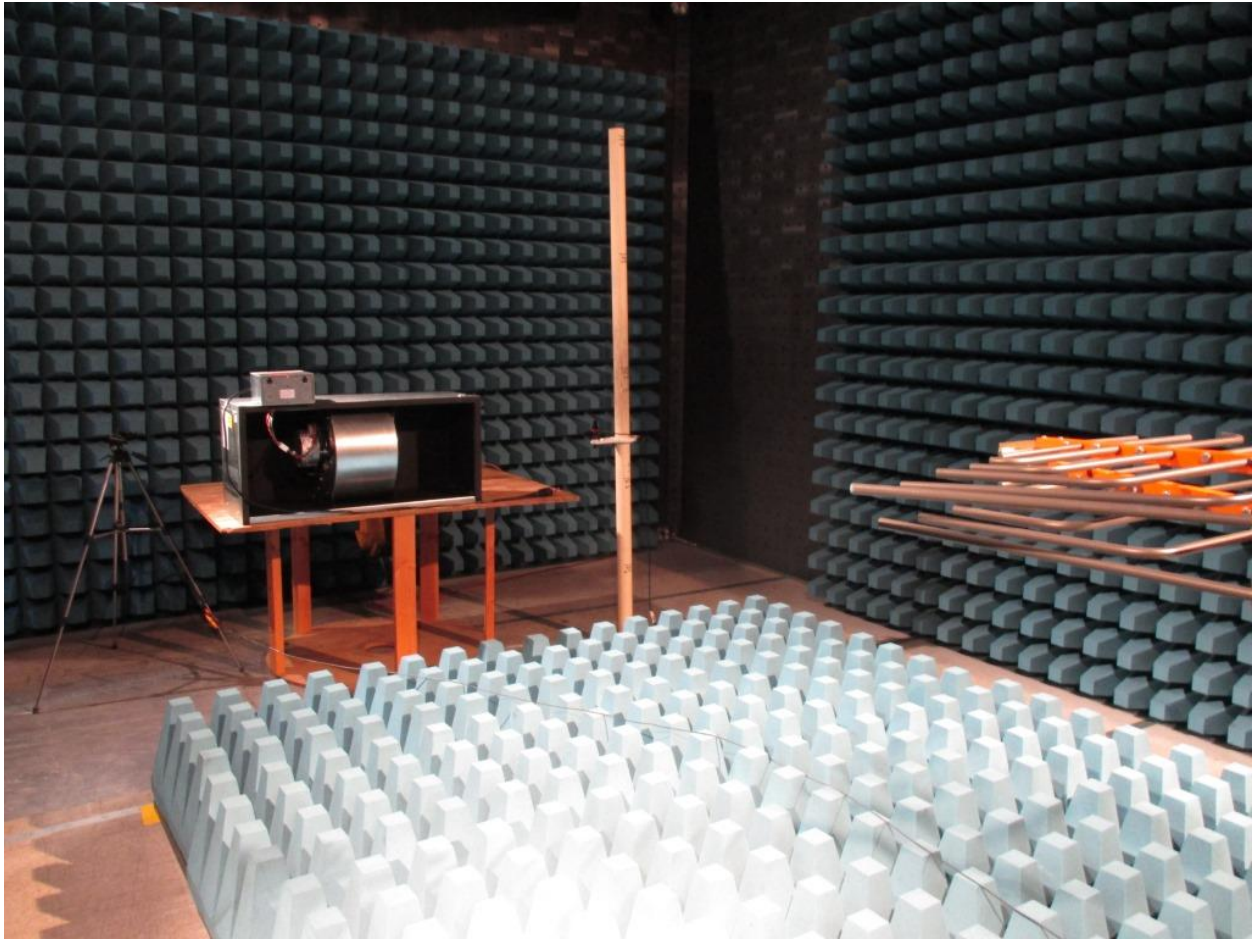
Figure 11-1 Radiated Immunity Test Setup
