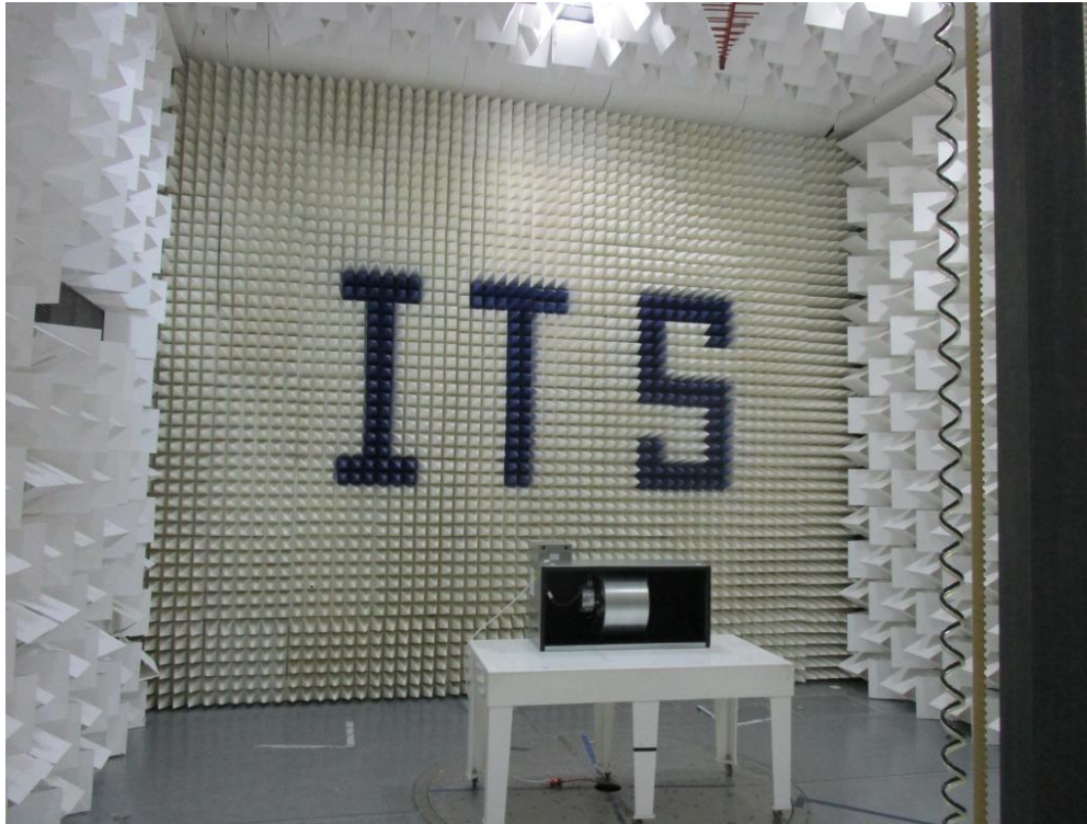
Figure 6-1 Radiated Emissions Test Setup Front
