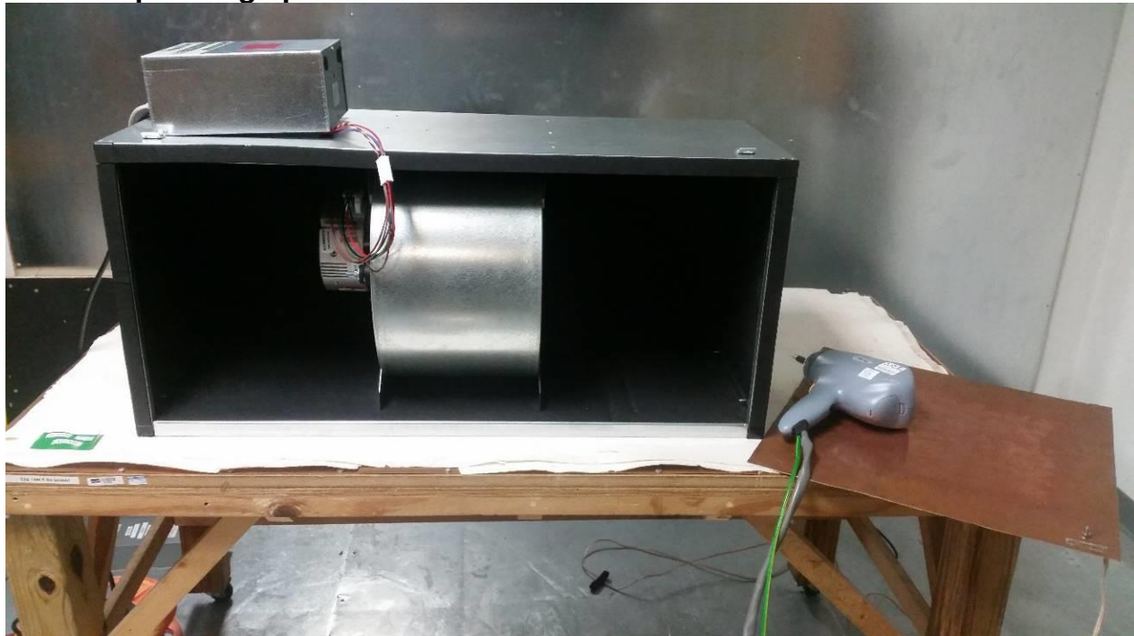
Figure 10-1 Electrostatic Discharge Test Setup
