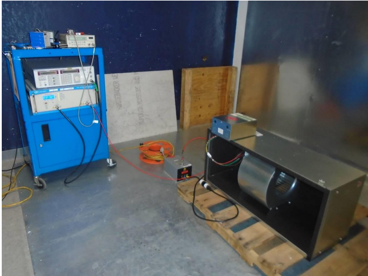
Figure 14-1 Conducted Immunity Test Setup
