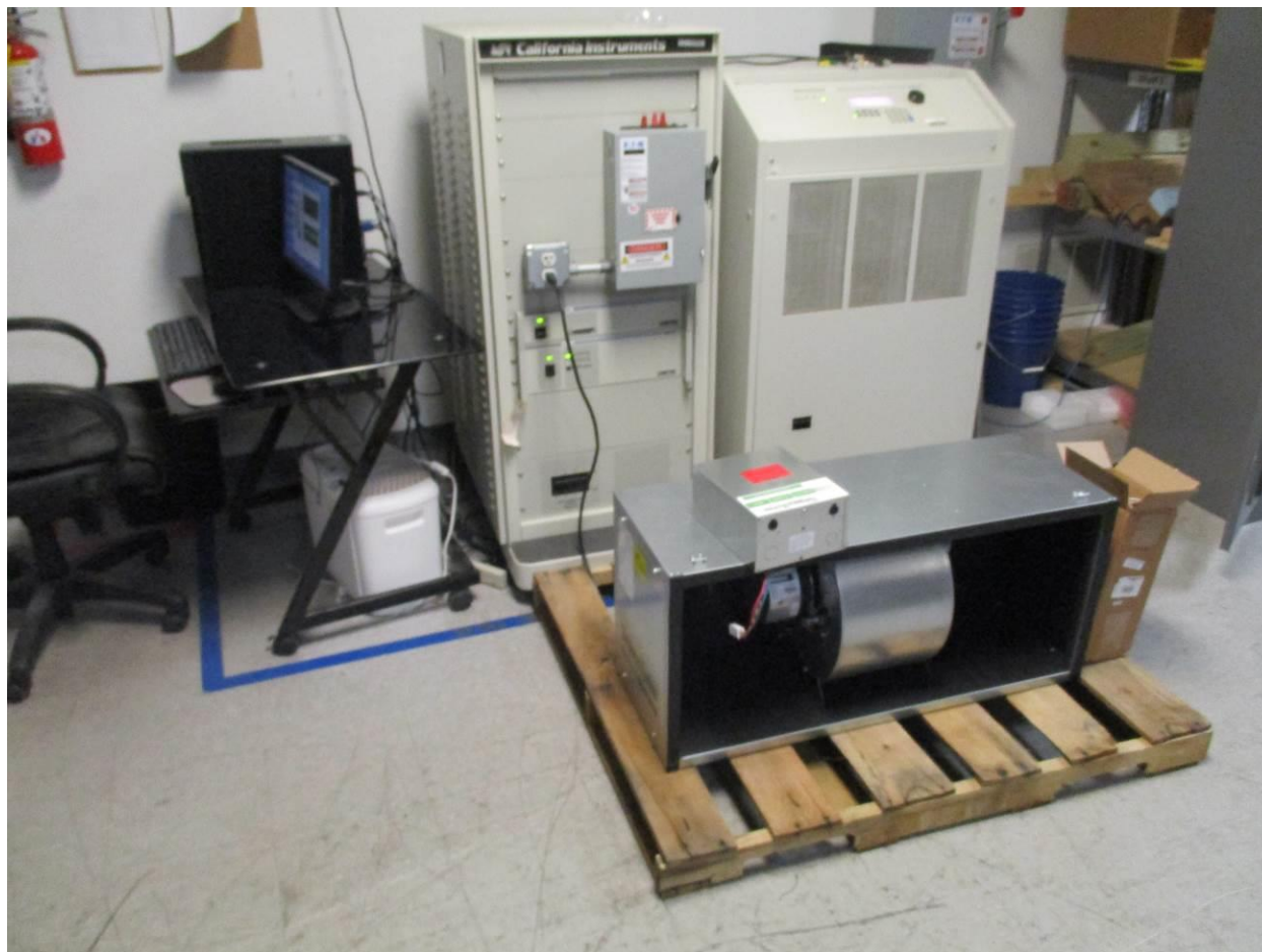
Figure 8-1 Harmonics Test Setup
