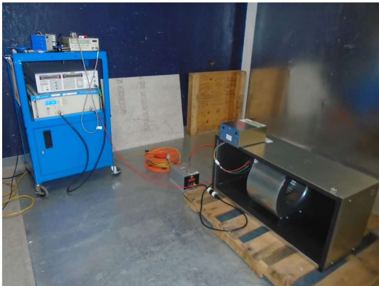
Figure 14-2 Conducted Immunity Test Setup
